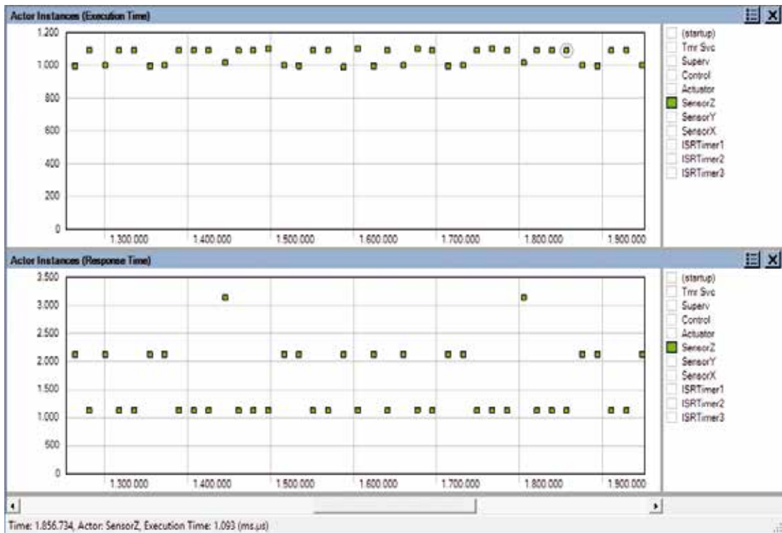
Figure 2. Plot showing variations in execution time (above) and response time (below), over time.
