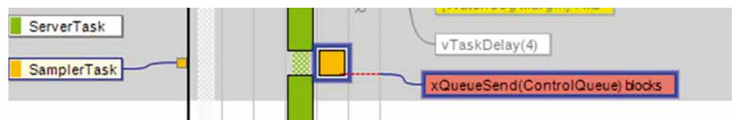
Figure 2. SamplerTask blocks on a send-to-queue operation.
