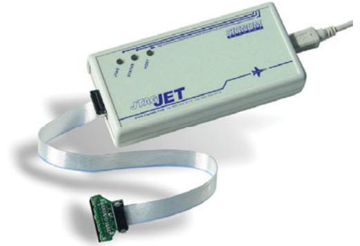
JTAGjet™ is a small, universal In-Circuit Debugger that connects to targets via the JTAG port. It is equipped with USB 2.0 high-speed port and on-board FPGA to achieve download speeds of up to 2MBytes/sec. JTAGjet-Trace™ has the same features as JTAGjet but contains ETM and PTM real-time trace capture logic with up to 18 MBytes of memory.
